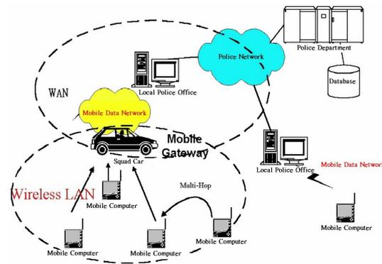
Fig.1 MPI S Architecture
