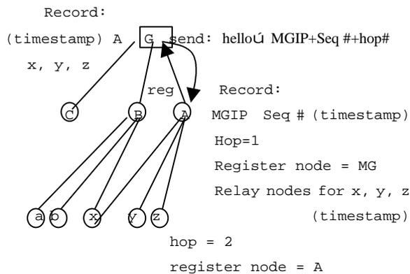
Fig.2 Multihop Architecture Control (Location Tracking)
